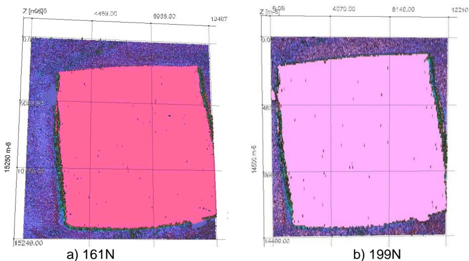
**Figure 3. 3D representation of reflectivity variation for the contact area between cylindrical roller with  $\Phi = 20mm, l = 11.4mm$  and a steel flat plate**
