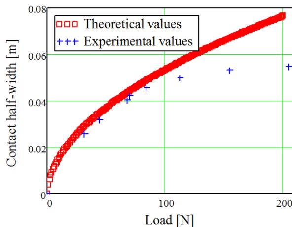
**Figure 8. Comparison between theoretical results obtained by Diaconescu and experimental measurements of contact half-width in a median region of contact area**
